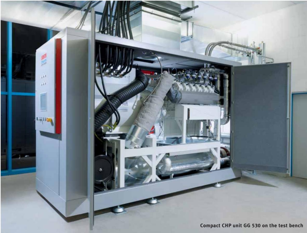
Compact CHP unit GG 530 on the test bench
